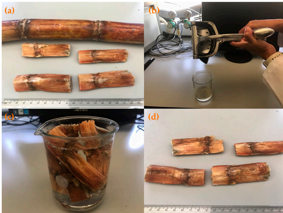
Figure 1. Process of preparing sugarcane samples to obtain bagasse. (a) Cutting sugarcane fragments, (b) juice extraction, (c) washing the sugarcane bagasse, and (d) dry fragments of sugarcane bagasse.
