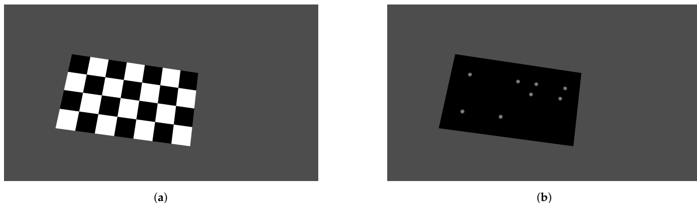
Figure 8. Example synthetic images of the checkerboard (a) and the bead array (b) targets, at the same relative position.
