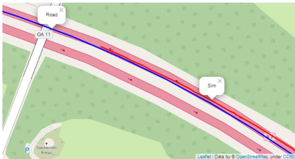
**Figure 5.** Vehicle trajectories from an exemplary real test drive (Road) and a simulation (Sim) at the validation scenario  $v_x = 169$  km/h and  $a_{y,ref} = 0.85 \cdot a_{y,max}$ , located on a OpenStreetMap of the German motorway A7. These trajectories of the vehicle’s center of gravity are shown at this point for illustration purposes, but not to derive detailed distances from the vehicle edges to the lines.
