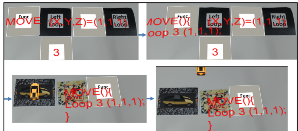
Figure 11. This is an example of controlling the 3D movement of the car. The markers will be read in a deep-first traversal mode—that is, read from left to right—and the column marker is read first when there is a column. The defined program is that the car moves with the 3D vector of (1, 1, 1) as a parameter and repeats this movement process 3 times.
