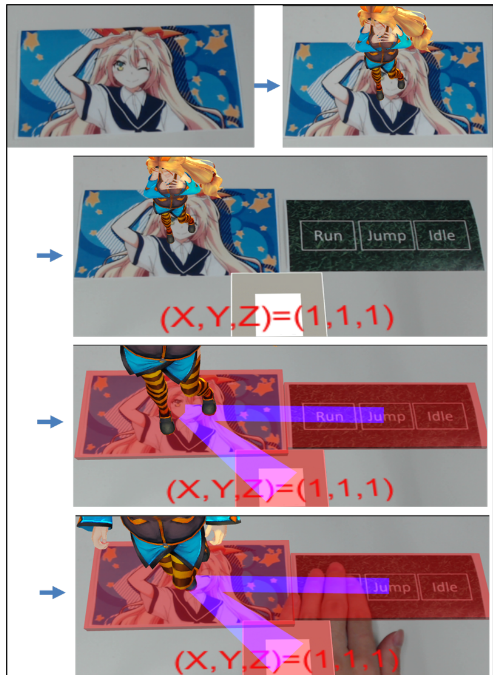
Figure 9. Using markers to control the size and movement of the avatar. The first image shows the avatar marker and the second image shows the avatar being superimposed on the avatar marker. The third picture shows the state of the markers before they are connected. After connecting the 3D vector marker and the avatar marker, the size of the avatar will be set to (1, 1, 1), as shown in the fourth picture. In the fifth picture, the user commands the avatar to run by clicking the control marker.
