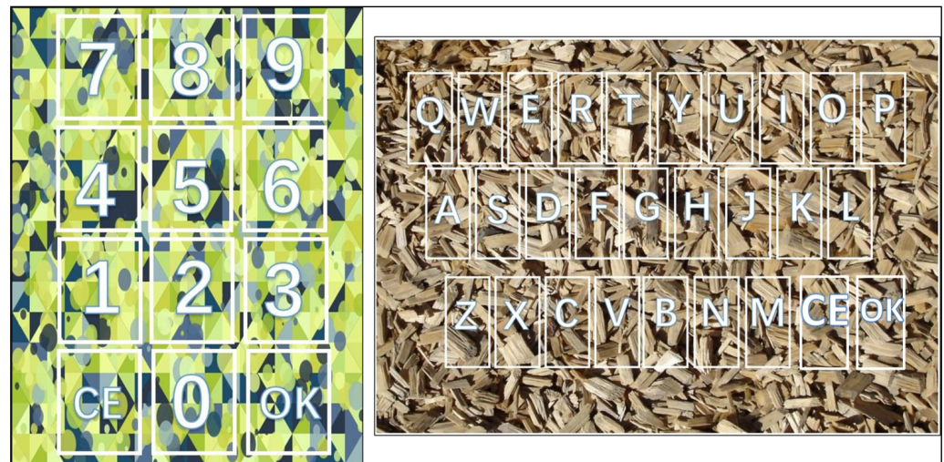
Figure 2. The figure shows two input markers. They can accept the corresponding input parameters through the user clicking on the marker. The content of each block represents the input information when the user clicks on the block. The CE button is used to delete the last number or character, and the OK button is used as a confirmation button.
