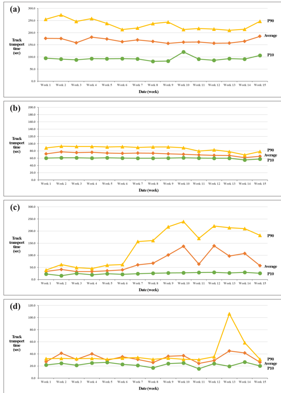
Figure 10. Time-series analysis results of stable and unstable transport routes in the study area using log data files per week (1–15 weeks): (a) beacon ID 19 to 1 (stable section); (b) beacon ID 11 to 10 (stable section); (c) beacon ID 3 to 5 (unstable section); (d) beacon ID 13 to 12 (unstable section).
