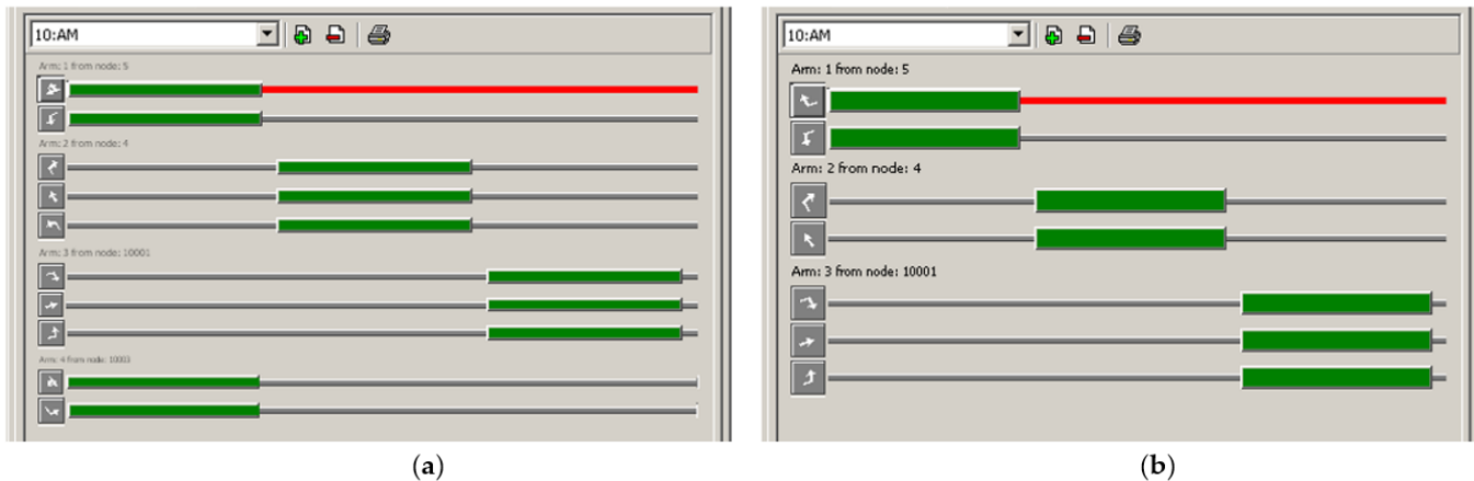
Figure 8. Illustration of the signal plan of the Palackeho–Stefanikova intersection for Variant A (a) and Variants B and C (b) (source elaborated by authors).
