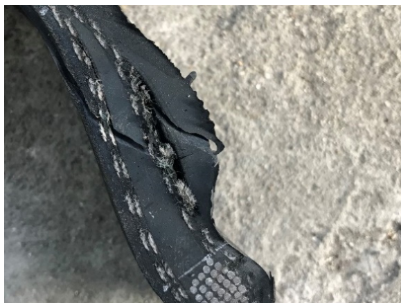
Figure 15. Failure section of tested tire.
