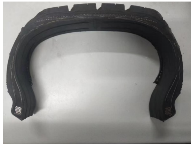
Figure 8. Cross-section of 175/75R14 tire.
