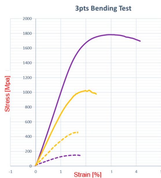
Figure 2. Diagram of three-point flexural strength on four different types of specimens.
