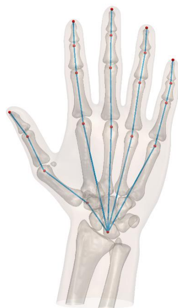
Figure 5. Linkage representation (blue) of a participant’s right hand by connecting the estimated joint centers (red).
