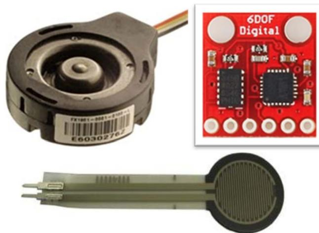
**Figure 3.** Force sensors, IMU sensor, and Interlink FSR sensor.
