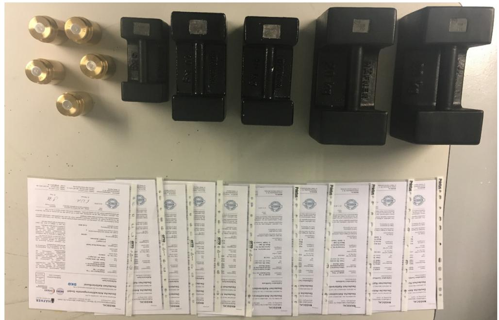
**Figure 13.** Calibrated weight set (Type: Class M2, calibration date 07/11/2019).
