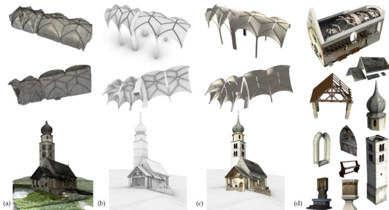
Figure 8. The scan-to-BIM process applied to the research case study: from digital photogrammetric model (a), NURBS model by GOGs (b), NURBS model (c) to HBIM textured objects (d).
