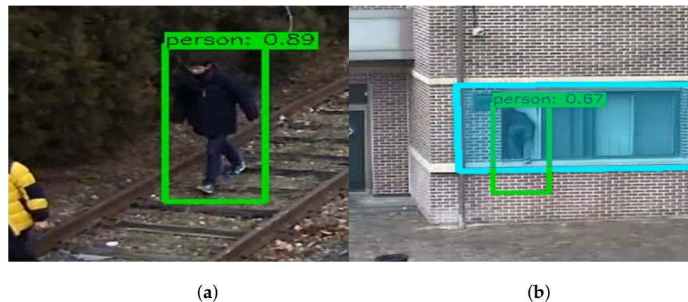
Figure 2. Two examples where the object goes out of image: (a) Objects that disappear from the outside of the image, (b) Objects that disappear within the image.
