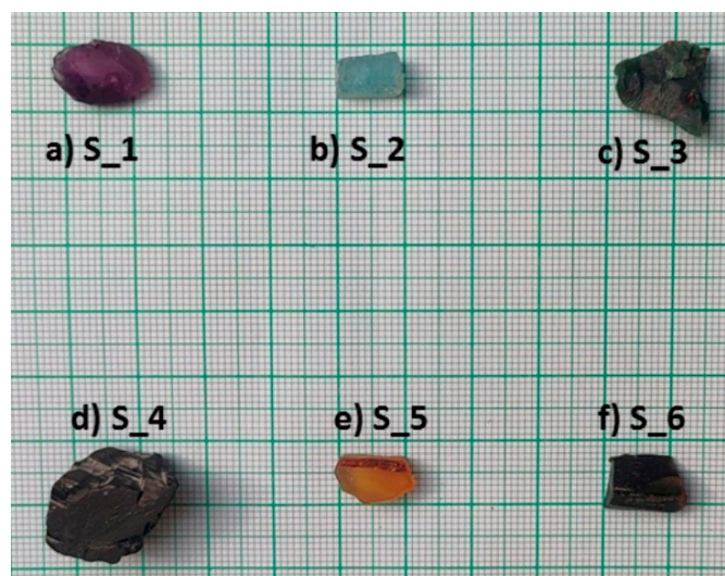
Figure 1. The gemstones analyzed during the present study are shown here. (a) Amethyst (S_1), (b) aquamarine beryl (S_2), (c) bloodstone (S_3), (d) diopside, (e) citrine (S_5), (f) enstatite (S_6).
