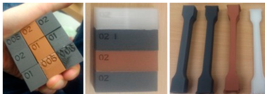
Figure 5. Samples for measuring surface roughness.
