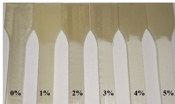
Figure 8. Photographs of ruptured specimens from PLA to 5% SEBS (left to right).
