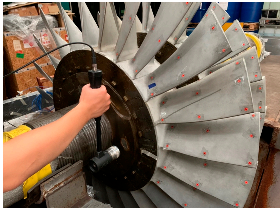
Figure 9. A typical X direction and the clock position of three o'clock meaning directly to the right of the excitation applied in modal testing of in-situ measurements.
