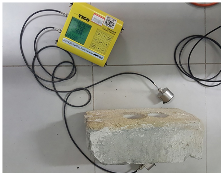
Figure 4. Ultrasonic test setup.
