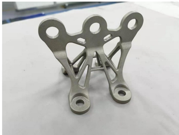
Figure 14. New bracket after 3D-printing with EOS M290.
