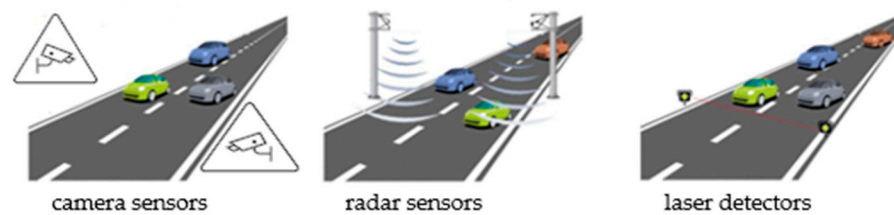
Figure 5. Non-intrusive sensors placed on the roadside at ground level or with a view of the road from above [40].
