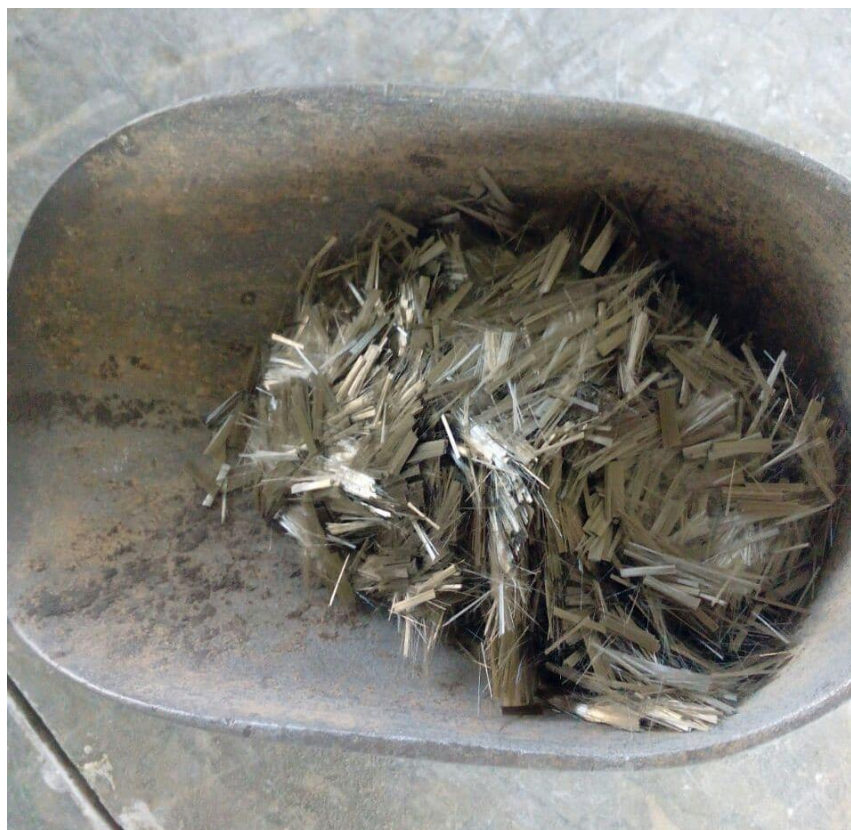
Figure 1. The basalt fibers (BFs) used in the production of the ECC mixture.
