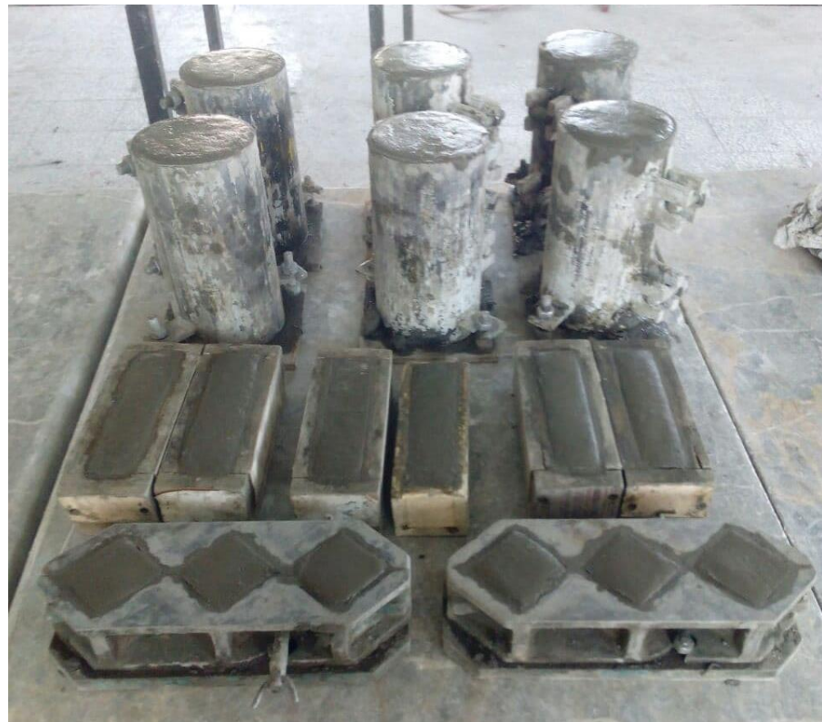
Figure 2. Molds after casting for tensile, flexural, and compressive strength tests from top downward, respectively.
