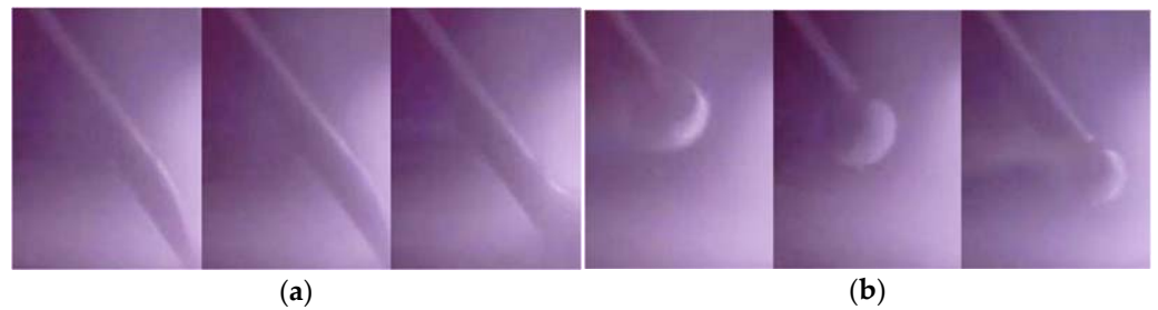
Figure 3. (a) Normal metal transfer shape; (b) abnormal metal transfer shape.
