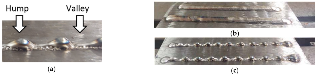
Figure 5. (a) Humping phenomenon (refer Nguyen et al. [49]); (b) normal bead; (c) abnormal bead.
