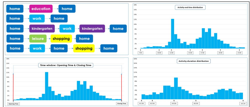
Figure 1. An overview of the model inputs. ( Top-left ): examples of activity-chains (home-based tours); ( bottom-left ): the activity-constraints represented by the time-window; ( top-right ): activity-end time distribution; ( bottom-right ): activity-duration distribution.
