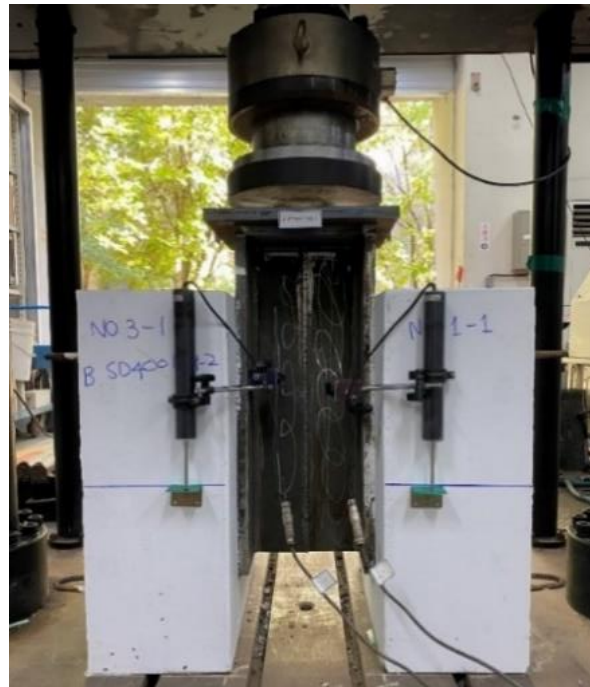
Figure 4. Test set-up of the push-out test.
