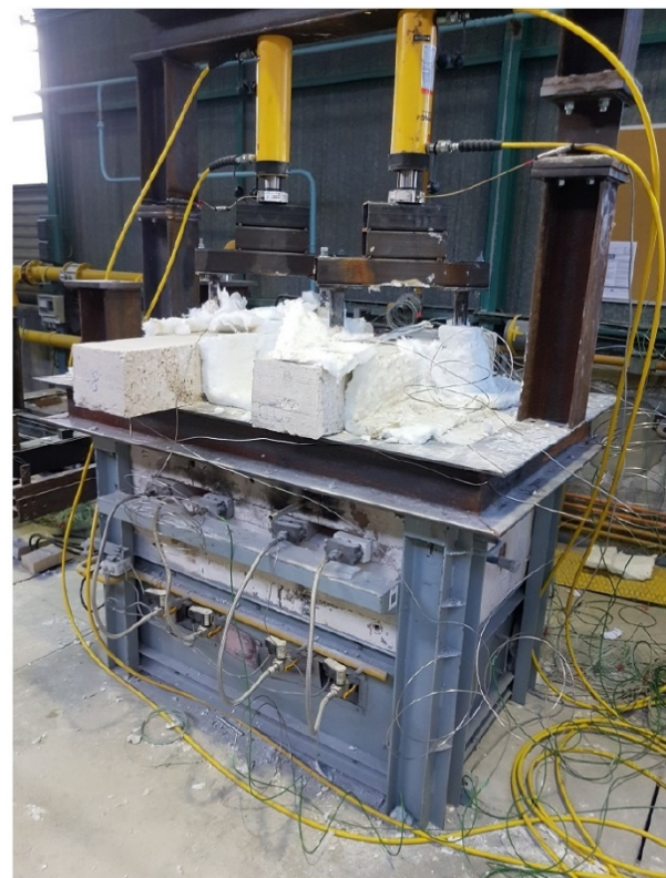
Figure 2. CSTB’s furnace and loading system for fire tests on bonded anchors [23].
