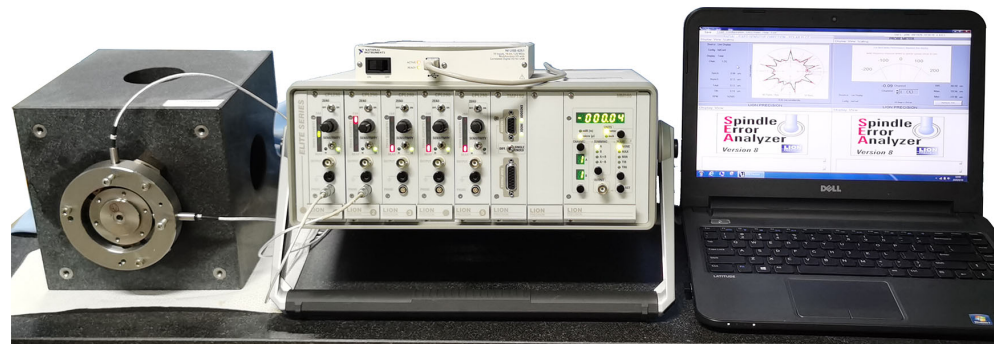
Figure 9. Test rig of spindle rotation error measurement.
