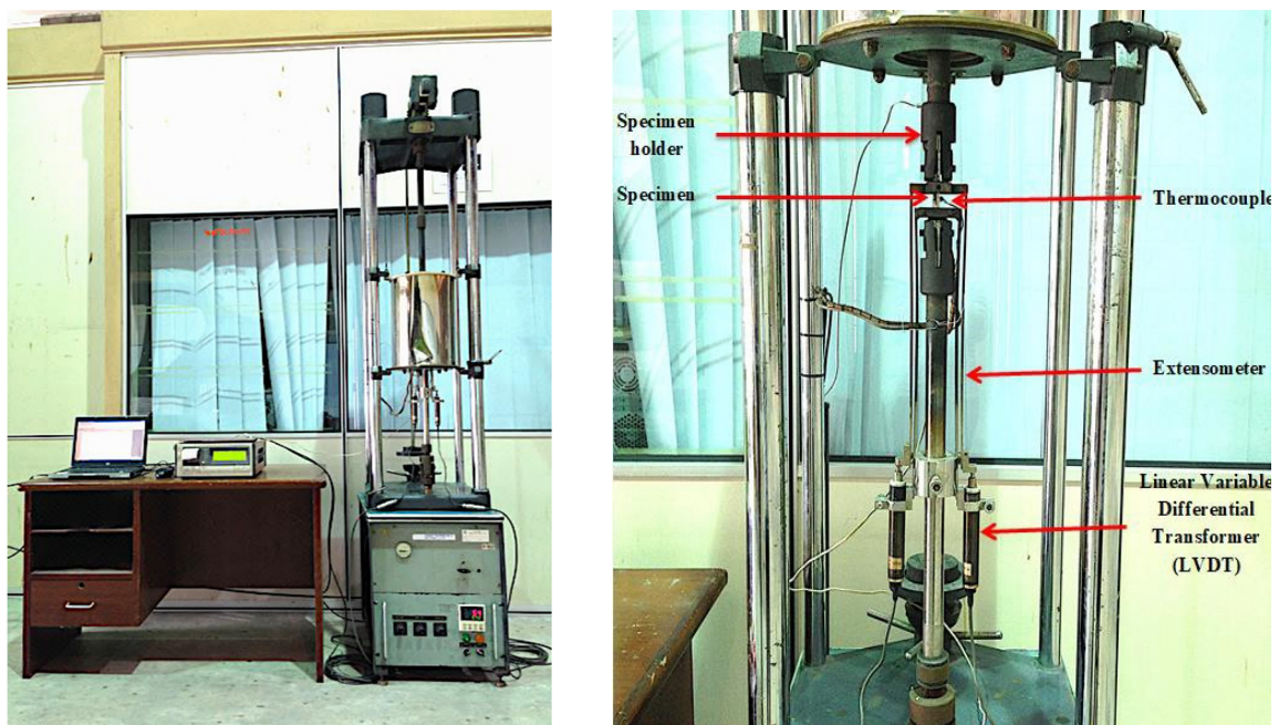
Figure S2. (A) High temperature creep machine and (B) Creep test setup for Fe-Ni-Cr alloys.
