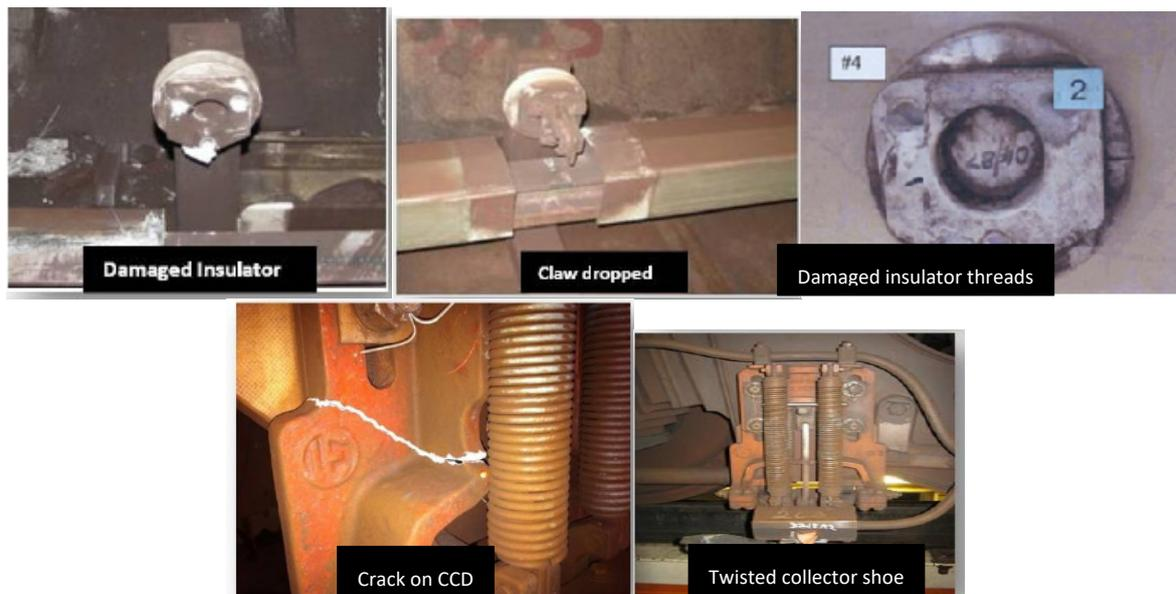
**Figure 10.** Nature of the damages and structural failures in third rail structure and current collector devices (CCD).
