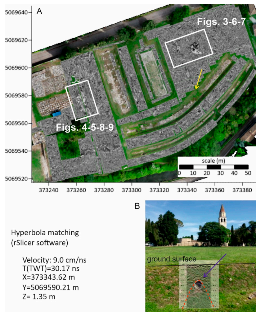
Figure 2. (A) Exemplary time-slice of the GPR data volume processed and the location of the areas reported in Figures 3–9; (B) Portion of a GPR profile crossing an outcropping pipe (its location is highlighted in A by the yellow arrow) and the result of the hyperbola fitting analysis.
