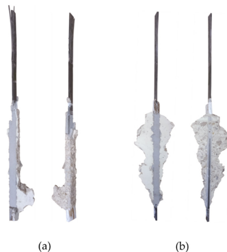
Figure 9. (a) S3-B-PSL-225-10-30 failure in the A-C interface; (b) S3-B-PSL-225-7.5-30 cohesive failure in the concrete.
