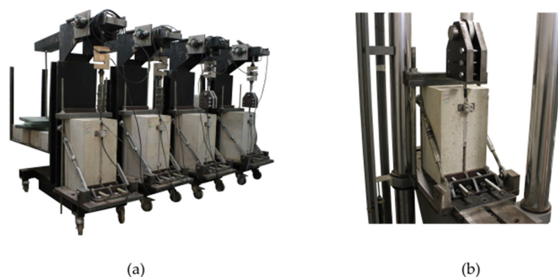
Figure 2. Set-up used for (a) sustained loading tests; (b) post-sustained loading tests.
