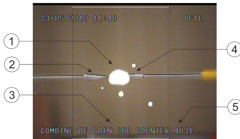
Figure 2. Image from camera screen with emission spectra signals originating from PDs: space of PD's formation (1); high voltage electrode (2); gain parameter (3); grounded electrode (4); number of counts (5).
