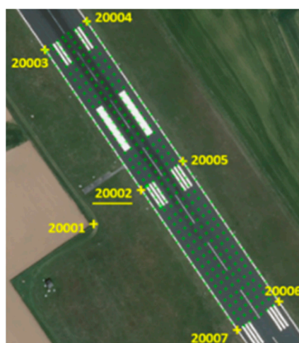
Figure 1. Basic (zero) geodetic network (yellow points) and NETWORK on the runway (green points) [56].
