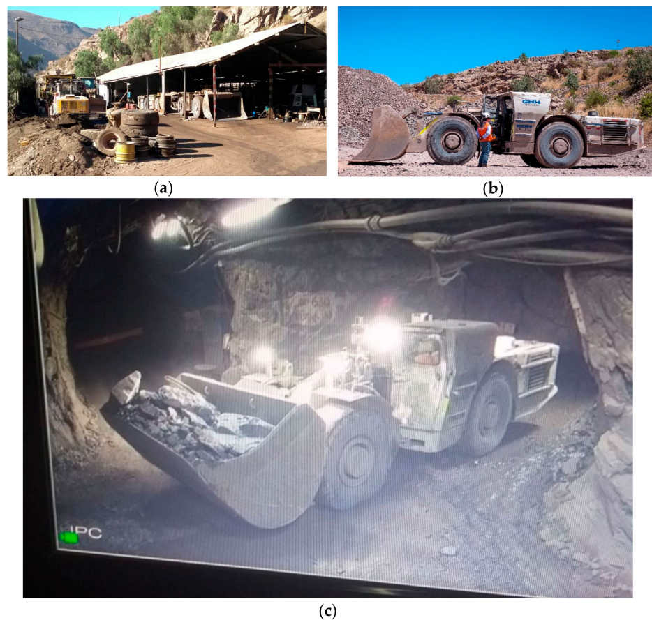
Figure 20. LHD machine and mining facility. (a) Mechanical workshop just outside the mine's main entrance; (b) LHD during surface tests; (c) LHD outside the test tunnel with an almost fully loaded bucket.
