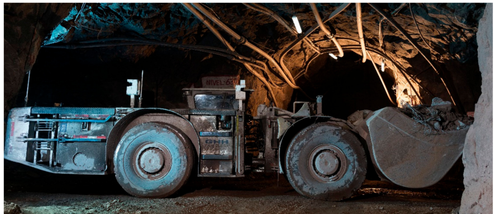
Figure 1. Full-scale LHD machine used during the test of the excavation algorithm.
