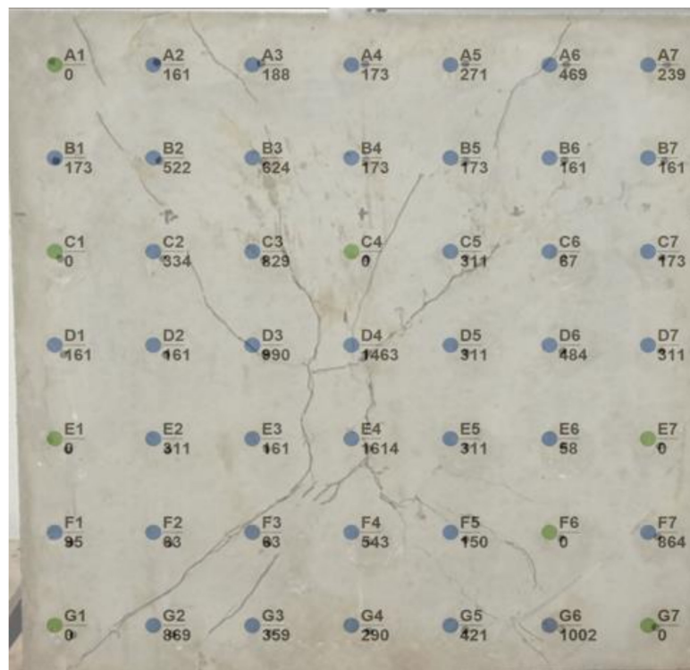
Figure 13. Schema of differences in measured velocities [ \text{m}\cdot\text{s}^{-1} ] of ultrasound waves for specimen A2_3 before and after blast load of 600 g TNT: acceleration (red color)—no point; no change (green color)—8 points; deceleration (blue color)—41 points.
