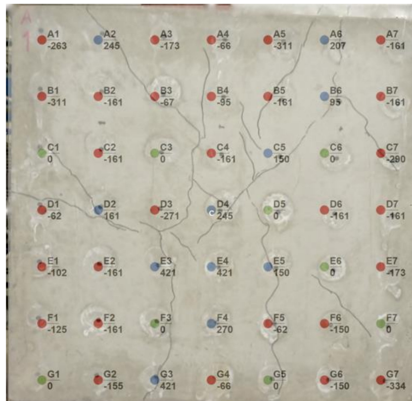
Figure 9. Schema of differences in measured velocities [ \text{m}\cdot\text{s}^{-1} ] of ultrasound wave for specimen A2_3 before and after blast load of 600 g TNT: acceleration (red color)–52.9% of points.
