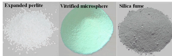
Figure 19. Inorganic materials for performance optimization of shotcrete.
