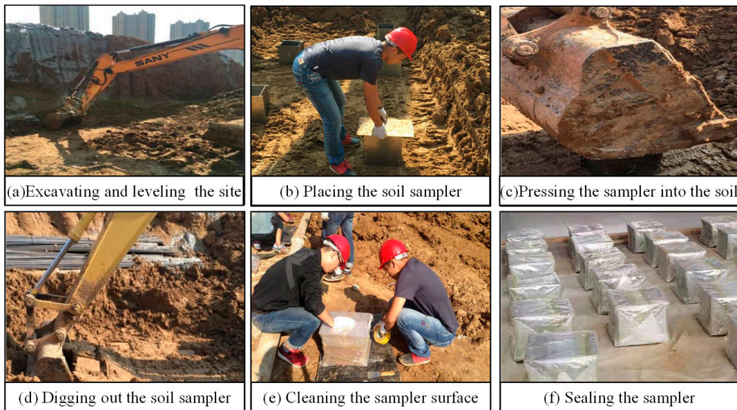
Figure 2. Soil sample from the undisturbed soil in the half-face pile test.
