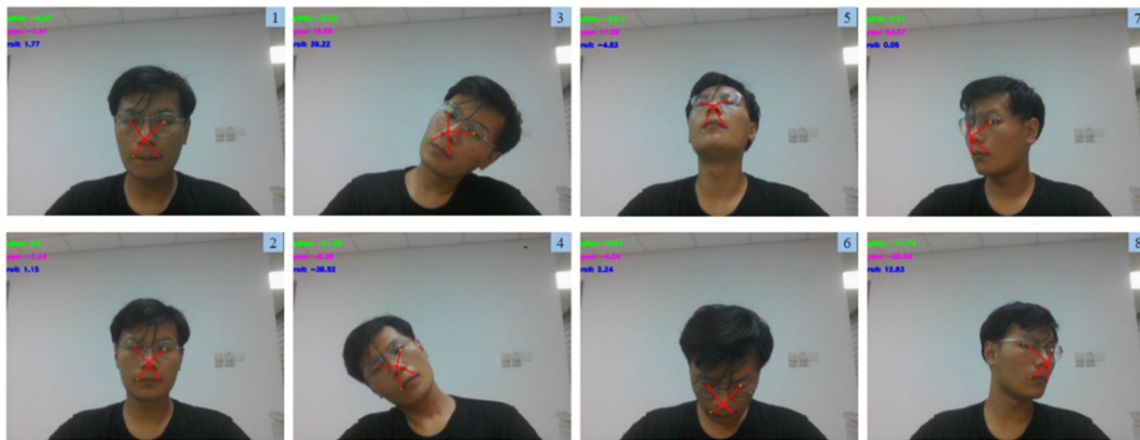
Figure 4. Results of head pose estimation by EPnP in a natural scene. 1 and 2 indicate that the head postures are normal. 3 and 4 indicate abnormal head rolling angles. 5 and 6 indicate abnormal head pitch angles. 7 and 8 indicate abnormal head yaw angles.
