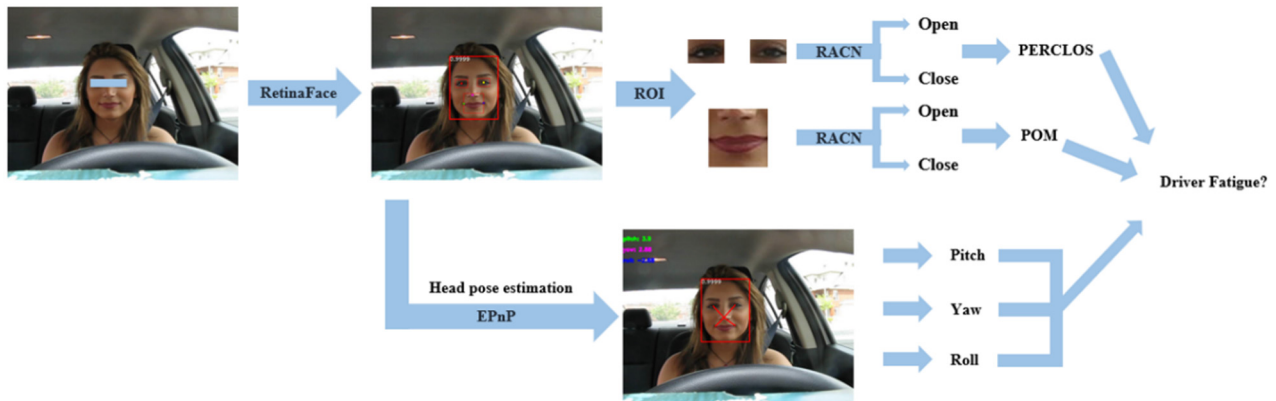
Figure 1. The overall structure of driver fatigue state detection.
