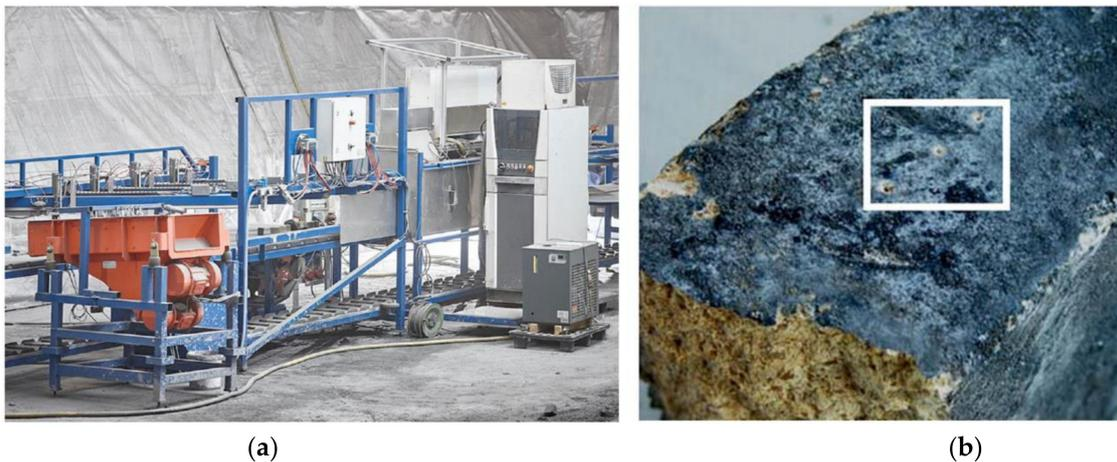
**Figure 15.** LIBS on-site measurement of spent refractory materials. (a) Demonstrator of a LIBS-based sorting machine (Photo: Orbix). Adapted from [461]. (b) End-of-life refractory brick with a modified surface layer. LIBS measurement spots marked with white rectangle (Photo: Fraunhofer ILT). Adapted from [208].
