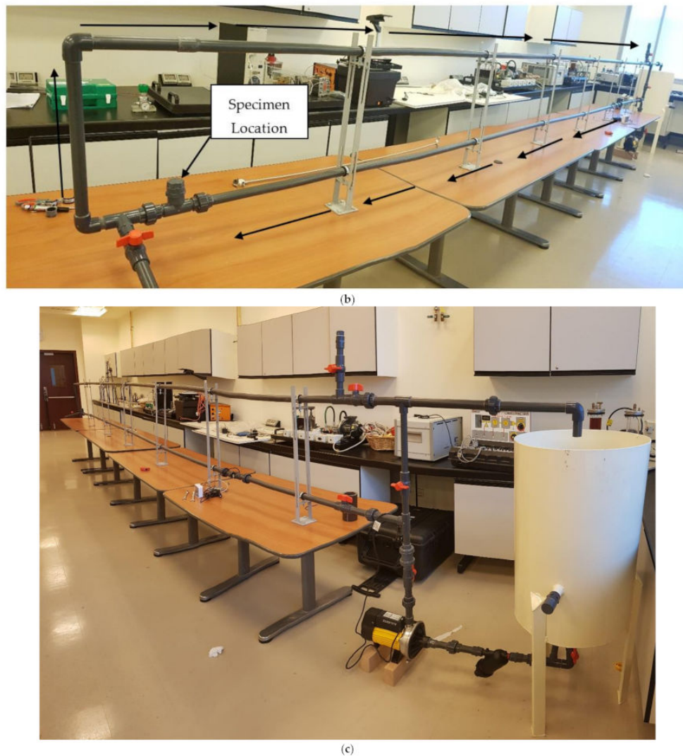
Figure 2. (a) Schematic diagram of the flow Loop, (b) flow direction and specimen location, (c) actual installed flow loop.
