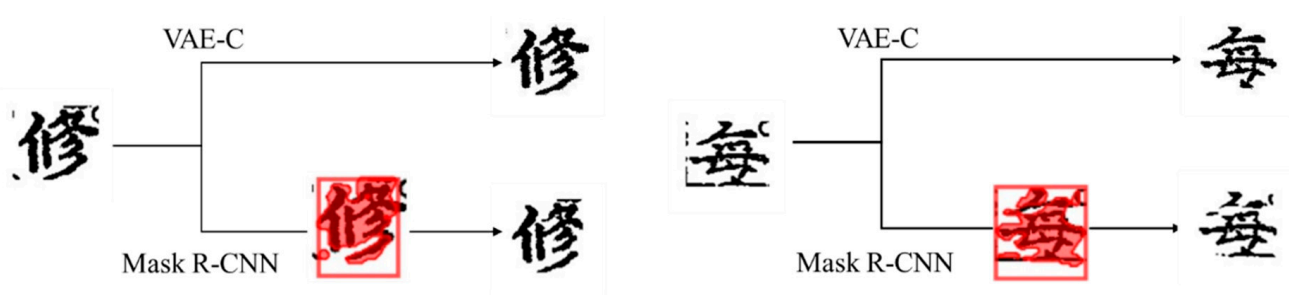
Figure 13. Comparison of the results of eliminating unnecessary objects by using the VAE-C model and Mask R-CNN (mask regions with convolutional neural networks).
