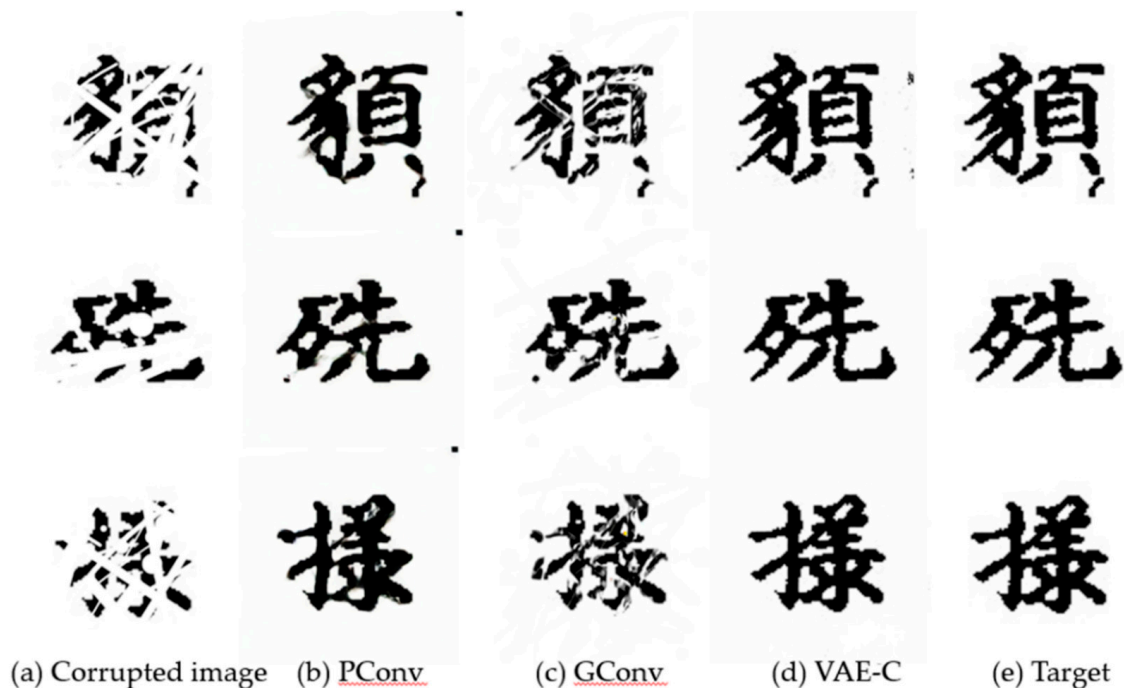
Figure 11. The results of restoring a corrupted image (a) that has corrupted the target image (e) using the partial convolution model (PConv) (b) [3], gated convolution model (GConv) (c) [4], and VAE-C model (d).
