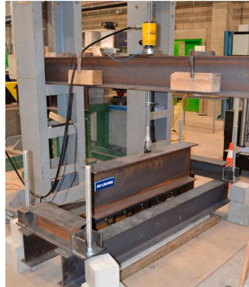
Figure 16. Pull-out tests on lattice girders: (a) results; (b) test setup.
