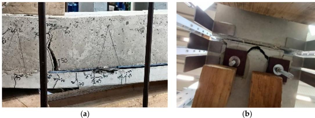
**Figure 11.** Observations from test C06: (a) typical crack pattern with formation of an overlap block and pull-out of the lattice girder before the end of the overlap reinforcement; (b) lower face of C06.
