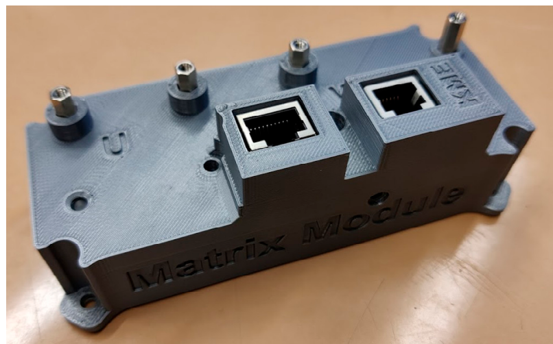
Figure 20. Assembled module with printed protection cover.
