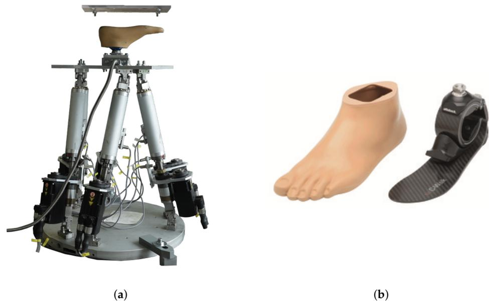
**Figure 6.** The transfer system and the experimental part are depicted. (a) The experimental setup consists of the prosthetic foot, the FTS, and the Stewart Platform. (b) The C-Walk foot 1C40 by Ottobock with silicone cosmesis (© by Ottobock).
