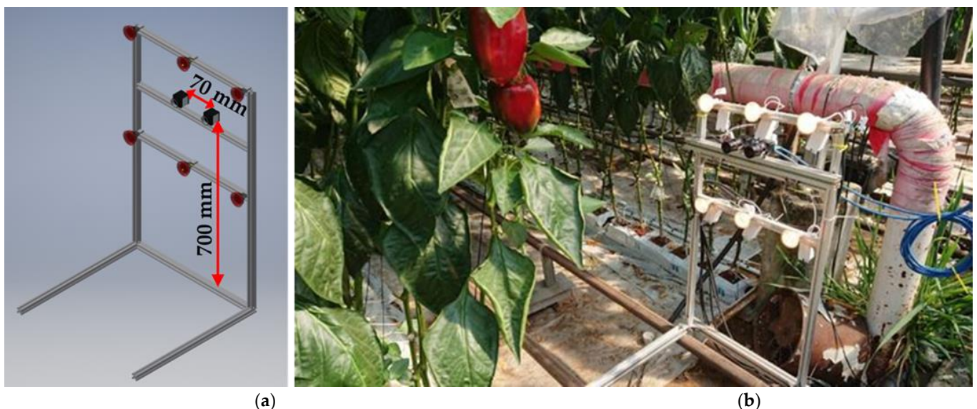
Figure 3. A structure for image acquisition (a) and image acquisition in the greenhouse (b).
