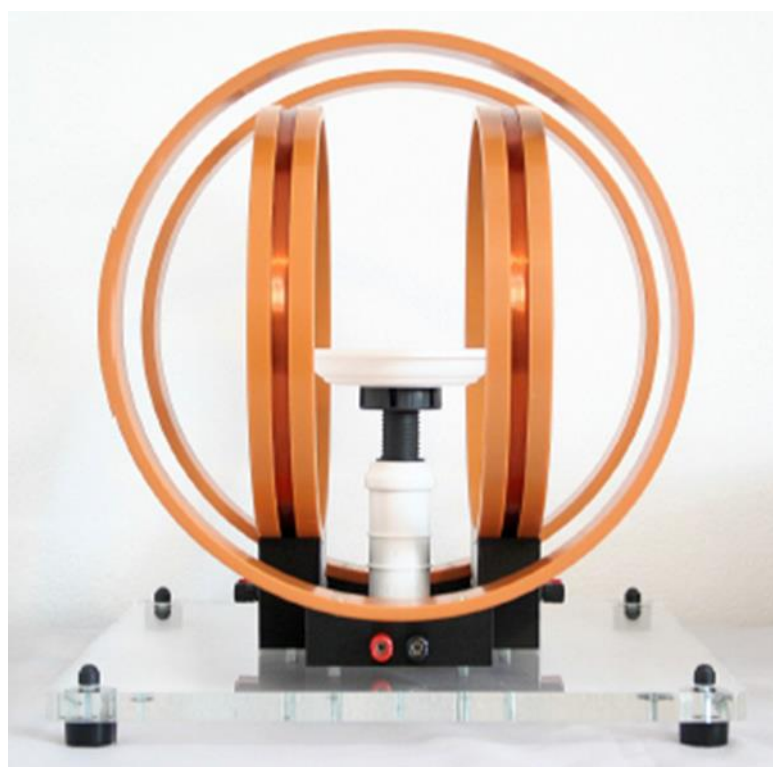
Figure 1. A set of coils for generating alternating magnetic fields (own study).
