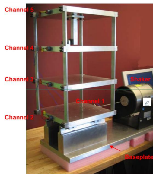
Figure 6. Position of accelerometer sensor installed structure.
