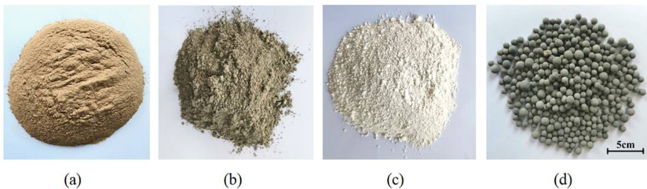
Figure 1. The raw materials: rock power (a), cement (b), lime (c) and FAC (d).
