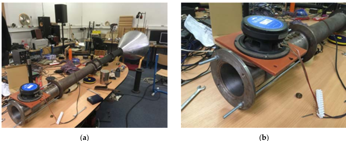
Figure 4. The measurement setup modification description. (a) Photo of full setup; and (b) the axis perpendicular side connection of LS.
