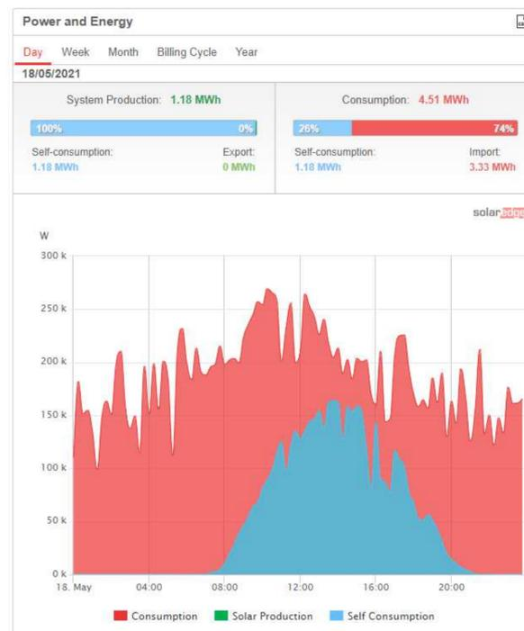
**Figure 12.** Screenshot of the monitoring portal showing the electricity consumption and production on one spring day (18 May 2021). The figure shows the 15-min average power in Watts for the consumption and PV production.
