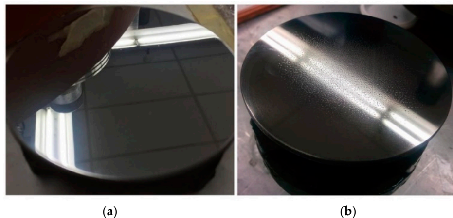
Figure 20. (a) Final Al mirror surface finish; (b) Final Ti mirror surface finish [30].
