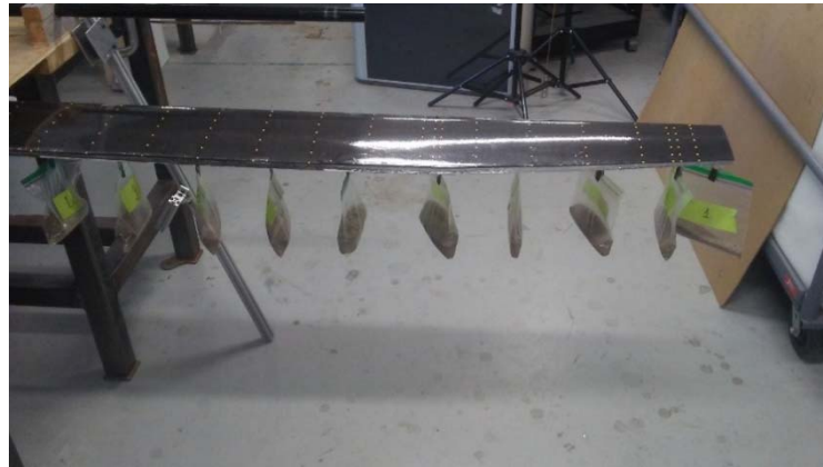
Figure 13. Morphing wing load test.
